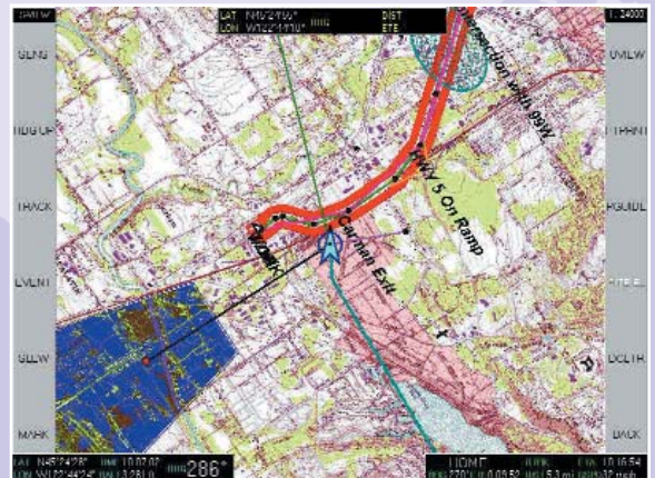
The Mission Management System's digital moving map showing the thermal imaging footprint in dark blue.
